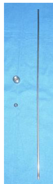
P0 cell (right) o-ring (upper left) Securing screw (lower left)
